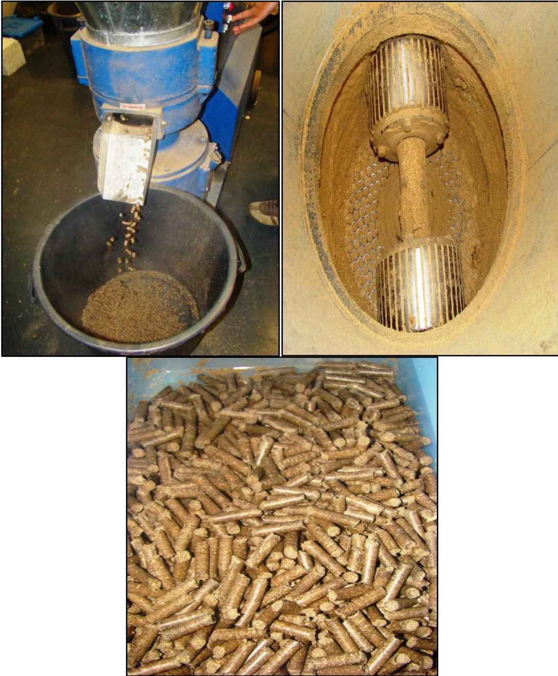
Pelletization of supports in pellet mill ZLSP300B R-Type
