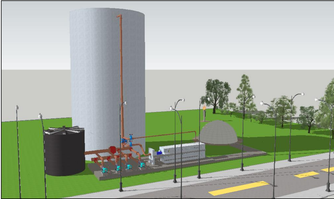
Figure 5.3 Isometric view of anaerobic reactor with membrane module coupled to recirculation line at real scale
